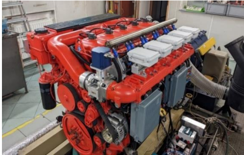
Fig. 18. Engine on the test stand in the Laboratory of ICEs of the Cracow University of Technology
