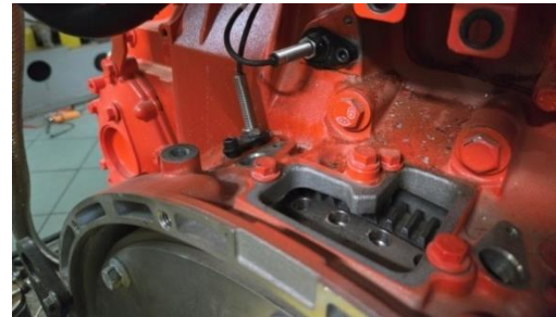
Fig. 15. Crankshaft and camshaft position sensors
