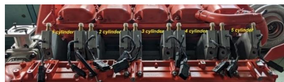
Fig. 13. Arrangement of gas fuel injectors in the engine (2 injectors per cylinder)
