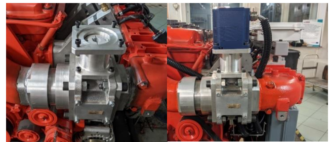
Fig. 7. Throttle module, during installation in the engine intake system (left), module with stepper motor controlling the throttle position
