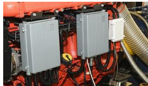
Fig. 16. Cassettes with the main engine control system
