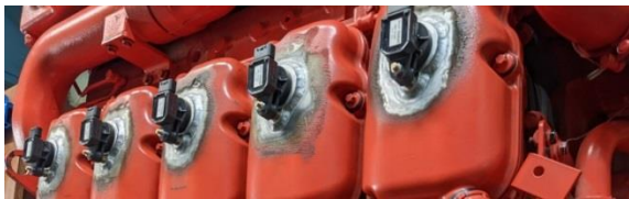
Fig. 14. Arrangement of ignition modules in the engine
