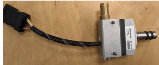
Fig. 10. Electronically controlled gas fuel injector
