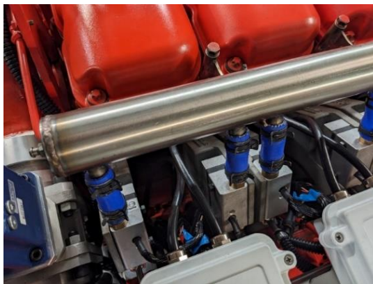
Fig. 9. A part of the fuel rail of the engine powered by gas fuels
