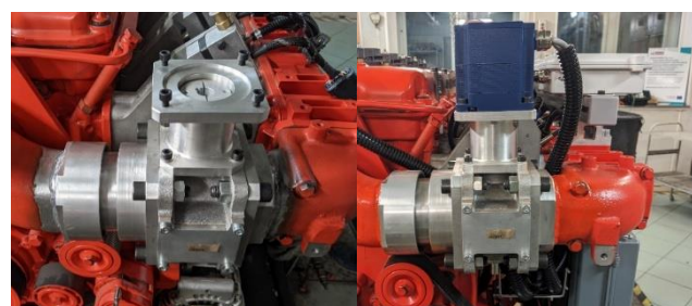
Fig. 7. Throttle module, during installation in the engine intake system (left), module with stepper motor controlling the throttle position
