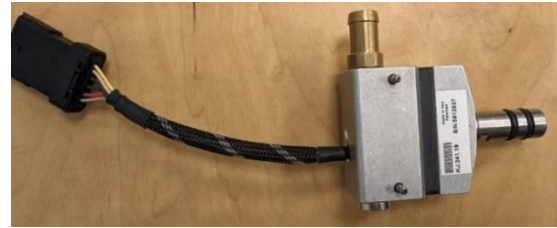
Fig. 10. Electronically controlled gas fuel injector
