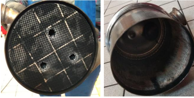
Fig. 4. Tested DPF filters with 3 holes and empty
