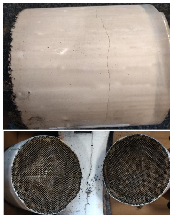
Fig. 17. The filter after removing it from the housing
