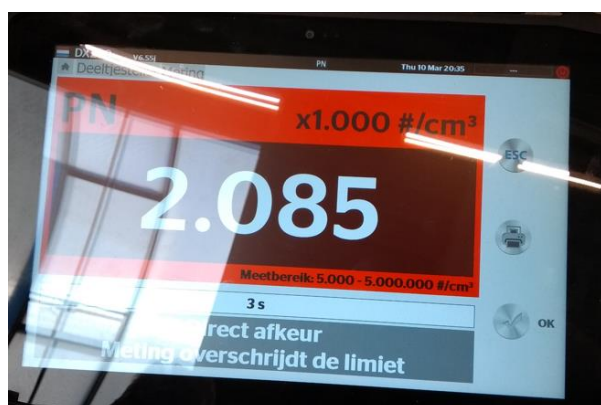
Fig. 8. PN measurement result on the Continental PNC display for the Peugeot 308 and for old OEM DPF
