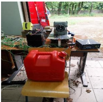
Fig. 5. Measuring station: A –test bench; B – GTM 120 engine; C – measuring probe
