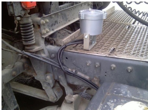
Fig. 5. a) View of the additional tank with a fuel microfiltration insert on the truck b) view of the tank with the KleanFuel insert with fuel lines [fot. Ł. Kubacki]
