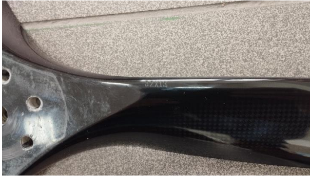
Fig. 18. Falcon 32/13 3-blade propeller – propeller geometry designation
