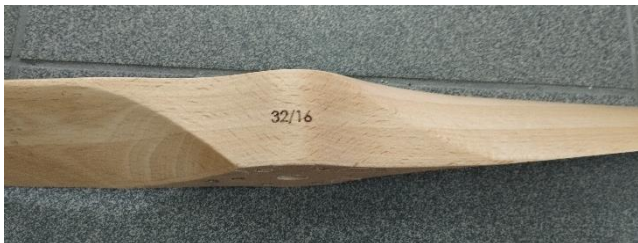
Fig. 10. Fiala 32/16 2-blade propeller – propeller geometry designation
