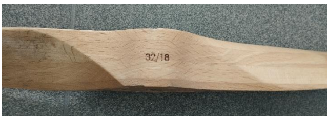
Fig. 12. Fiala 32/18 2-blade propeller – propeller geometry designation
