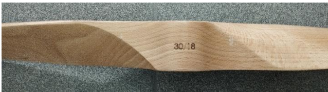
Fig. 8. Fiala 30/18 2-blade propeller – geometry designation
