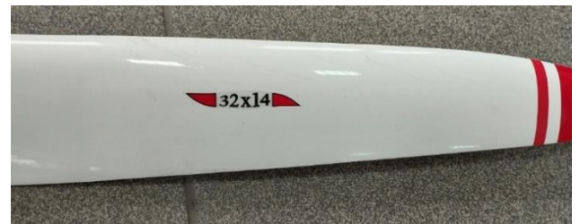
Fig. 14. Biela 32/14 3-blade propeller – propeller geometry designation
