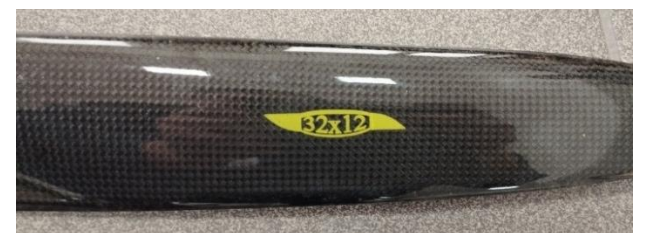
Fig. 16. Biela 32/12 3-blade propeller – propeller geometry designation
