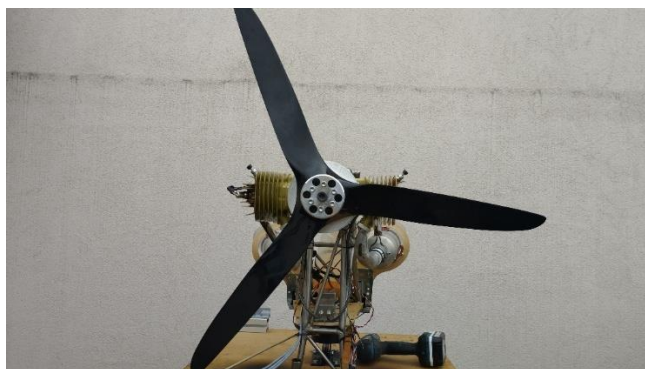
Fig. 5. 3-blade propeller made of carbon fibre
