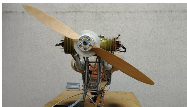
Fig. 6. 2-blade propeller made of wood
