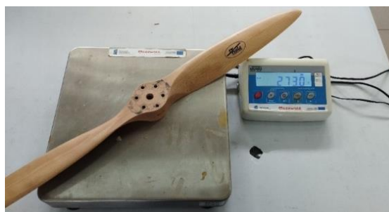
Fig. 19. Exemplary measurement of propeller mass using WLC 30/F1/K scales – result 273.0 g
