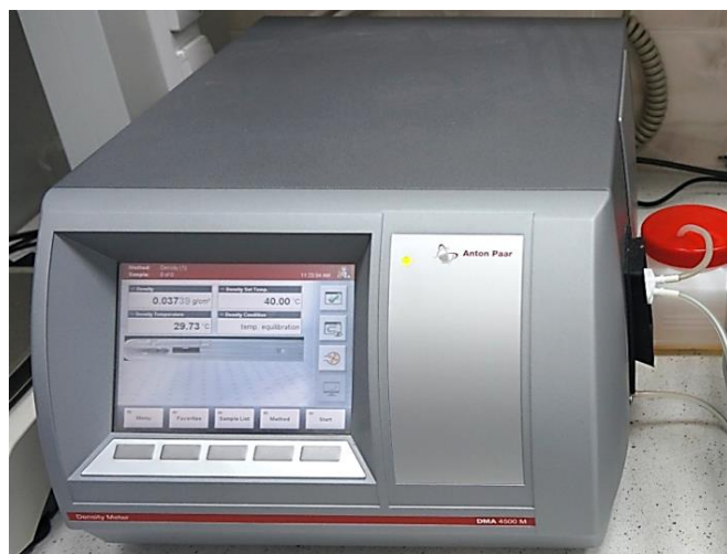
Fig. 1. DMA 4500 M apparatus for density determination
