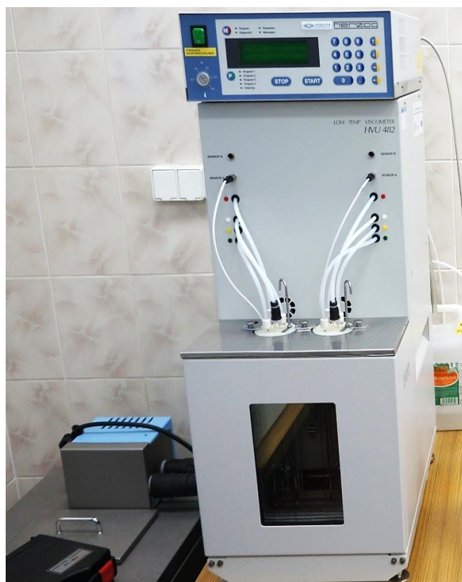
Fig. 2. HVU 482 apparatus for determining kinematic viscosity
