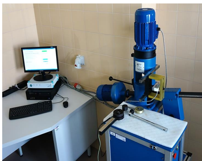
Fig. 3. View of the test stand for lubricity evaluation with the T-02U four-ball apparatus
