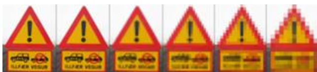
Fig. 8. Effect of decreasing resolution using the example of a traffic sign ( 480 \times 650/72 \times 96/36 \times 48/24 \times 32/18 \times 24/12 \times 16 ) [23]
