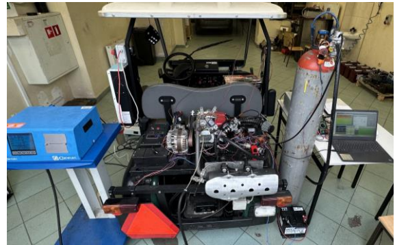
Fig. 6. Range extender test stand
