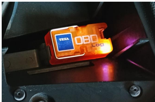
Fig. 2. TEXA OBD Log used to collect data in road tests
