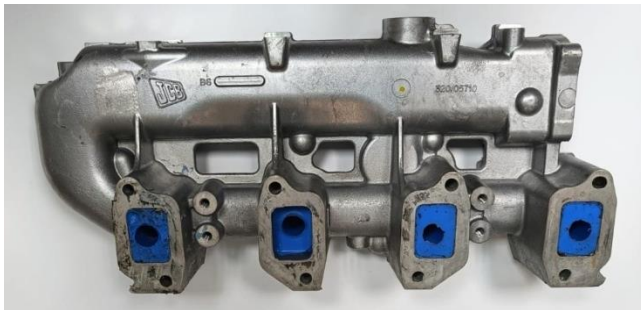
Fig. 2. Intake manifold filled with molding silicone
