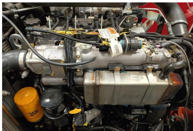
Fig. 1. Intake manifold of JCB 444 TA4i-81 I1 engine
