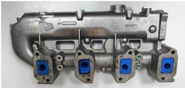
Fig. 2. Intake manifold filled with molding silicone
