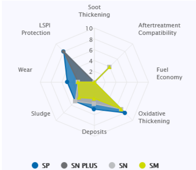
Fig. 1. API spark ignition standards [13]
