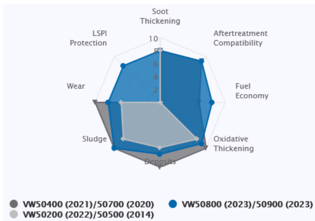
Fig. 9. Comparison of VW specs [13]
