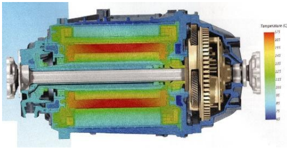
Fig. 7. Temperature inside the bus traction engine without an internal liquid cooling circuit [2]
