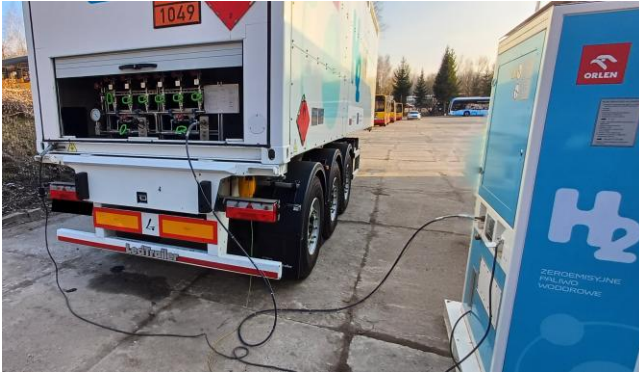
Fig. 2. Mobile hydrogen refueling station
