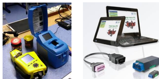
Fig. 6. Tribodiagnostic devices Q-1000, Q-3050 and EOBd – Gutmann Mega Macs PC
