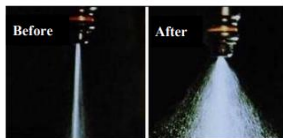
Fig. 1. Fuel nozzle operation before and after the use of additives (illustrative photograph) [2]
