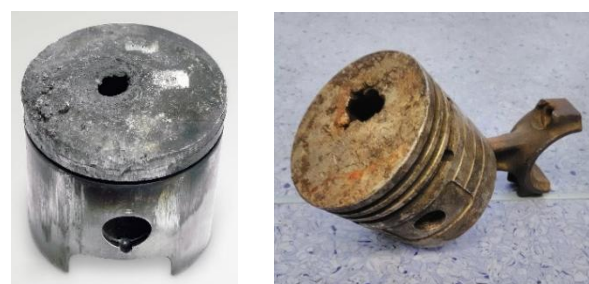
Fig. 2. Damaged pistons (illustrative photograph)
