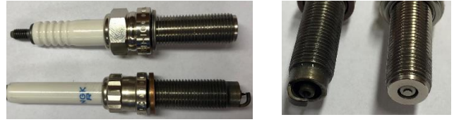
Fig. 1. View of SPF and SPJ spark plugs used for the engine tests
