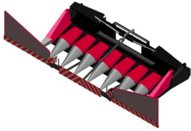
Fig. 7. Model of transport cover hooked on the header (unfolded position)
