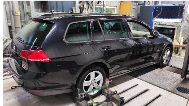
Fig. 3. Test vehicle evaluated under the NEDC driving cycle on a chassis dynamometer
