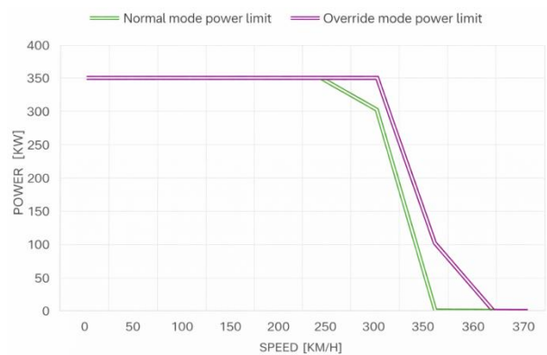
Fig. 16. Differences between the new engine modes [26]
