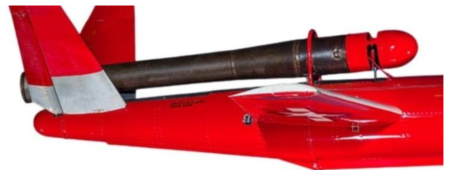
Fig. 3. McDonnell XPJ40-MD-2 valved pulse jet engine with side air entry (McDonnell TD2D Katydid air target [24])
