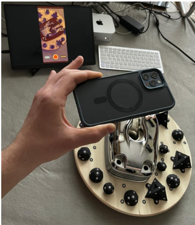
Fig. 4. Scanning of the valve cover using True Depth technology. The iPhone was held in hand with the display facing the object being scanned, while the portable external monitor displayed image from the RGB camera and the TrueDepth sensor
