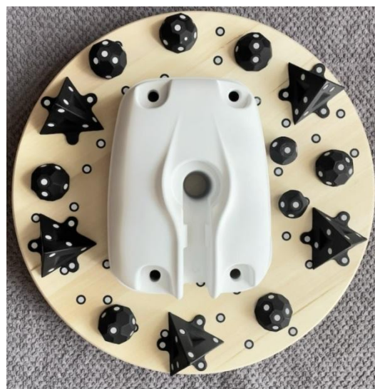
Fig. 3. Spray-coated valve cover lying on a rotating table
