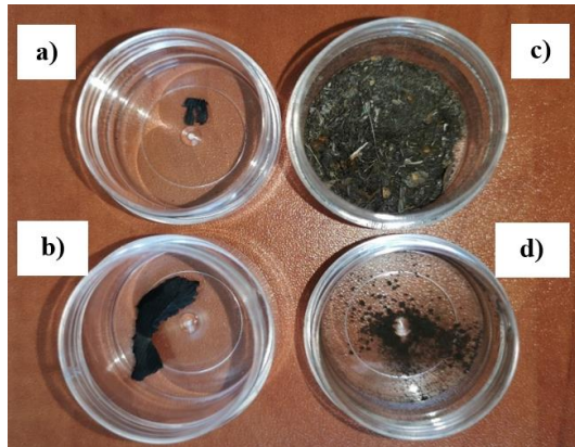
Fig. 9. Dust samples: a), b) passenger car tire sample, c) dust sample collected from the air filter, d) dust sample from the braking system
