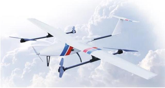
Fig. 5. Example of VTOL UAV platform [23]
