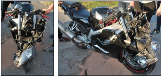
Fig. 2. Illustration of the deformation of the Honda CBR600F motorcycle
