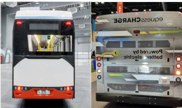
Fig. 18. EU and NA lights layout
