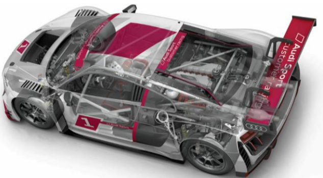
Fig. 3. Production-based Audi R8 LMS GT3 with a series-derived V10 and race-modified suspension [4]
