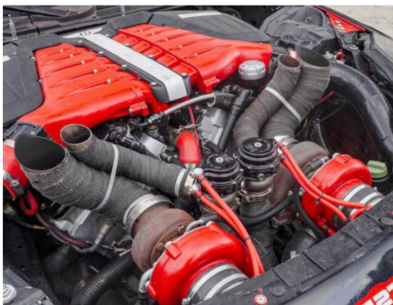
Fig. 6. Drift-spec Nissan 350z (a) with W12 high-performance engine (b)
