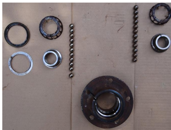
Fig. 8. Elements of the left rear wheel bearing: rolling balls on the right display characteristic signs of fatigue-related surface damage
