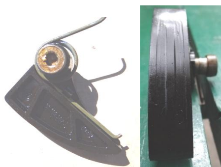
Fig. 6. Guide rail of the oil pump drive chain, identified as an original component from the vehicle's production period. Distinct frictional wear marks are visible on the sliding surface
