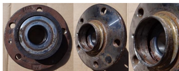
Fig. 7. Left rear wheel bearing removed from the vehicle, showing leakage of lubricating grease with a dense, viscous consistency typical of long-term exploitation
