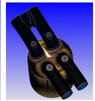
Fig. 3. Pictorial view of Siamese port GDI engine geometry
